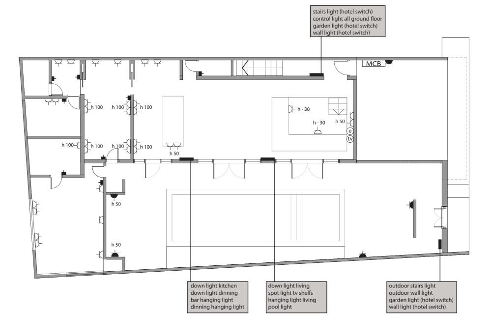
\* All light switches high is 100 cm from the floor level, 15 cm from the end of the wall except bedsided swithes
